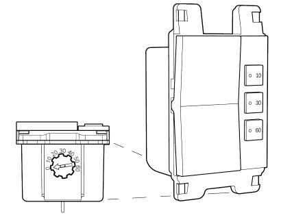
This Simple Ventilation Timer Switch is designed to monitor and control the operation of the bathroom exhaust fan and delivers a precise amount of fresh air ventilation throughout the day, automatically. Using the dial located on the side of the switch, the user can adjust the 'ventilation' setting. When used in conjunction with the countdown timer buttons, both timers ensure that the bathroom is properly ventilated at all times.
